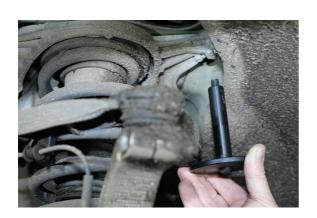
Install the FUCA (front upper control arm) ride height tool on to the mounting hole.
